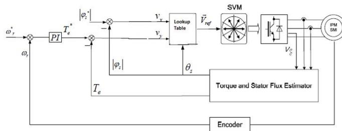
Figure 3. Conventional DTC Applied to PMSM
