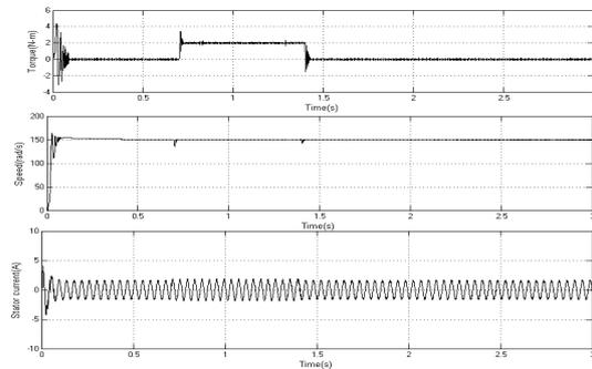
Figure 17. Conventional DTC: Load Torque of 2 Nm Applied at 0.7 sec and Removed at 1.4 sec
