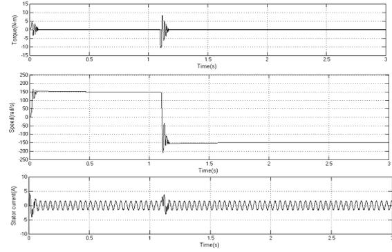
Figure 16. Proposed DTC: Transients during Speed Reversal
