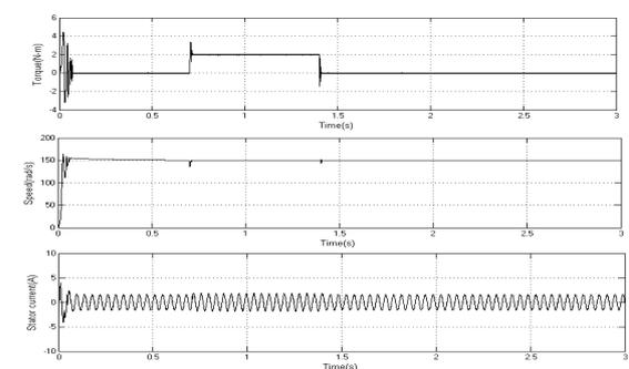
Figure 18. Proposed DTC: Load Torque of 2 Nm Applied at 0.7 sec and Removed at 1.4 sec
