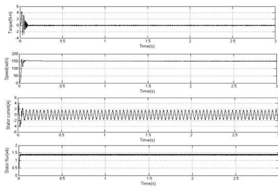
Figure 11. Conventional DTC: No Load Starting Transients
