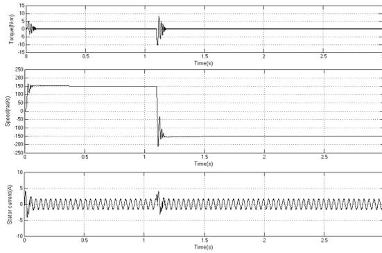
Figure 15. Conventional DTC: Transients during Speed Reversal
