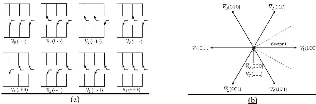
Figure 2. (a) Switching states of 2-level Inverter, (b) Voltage vectors applied to Inverter
